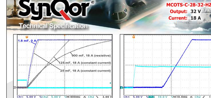
Figure 7: Hi-Cap Startup Waveform, input voltage pre-applied. Ch 1: Vout, 1.8 mF, no load (5 V/div); Ref 1: 25 mF, 18 A CC load; Ref 2: 125 mF, 18 A CC load; Ref 3: 900 mF, 18 A CR load; Ch 2: ON/OFF (5 V/div). Timescale: 400ms/ div.
