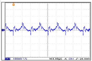
Figure 10: Output Voltage Ripple, Vout, at nominal input voltage and rated load current (100 mV/div). Load capacitance: 1 µF ceramic and 100 µF electrolytic capacitors. Bandwidth: 20 MHz. Timescale: 4.00µs/div. See Figure 13.
