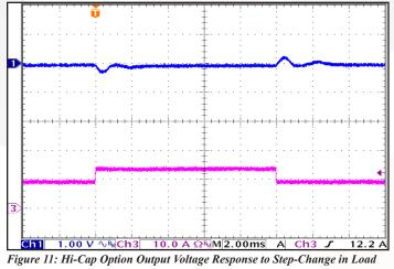
*Current,* (50%-75%-50% of *Iout(max); dI/dt* = 10 *A/µs*). *Load capacitance:* 1 µF ceramic and 5 mF electrolytic capacitors. Ch 1: AVout (1 V/div); Ch 3: Iout (10 A/div). Timescale: 2.00ms/div.
