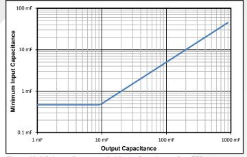
Figure 15: Minimum Recommended Input Capacitance, low-ESR capacitors preferred. See "HiCap App Section" for additional information.
