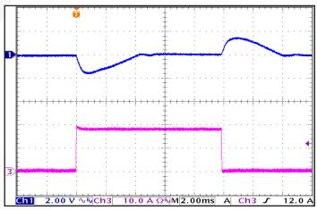
Figure 12: Hi-Cap Option Output Voltage Response to Step-Change in Load *Current,* (0%-100%-0% of *Iout(max)*;  $dI/dt = 10 A/\mu s$ ). Load capacitance:  $1 \mu F$ ceramic and 5 mF electrolytic capacitors. Ch 1:  $\Delta Vout$  (2 V/div); Ch 3: Iout (10 A/div). Timescale: 2.00ms/div.
