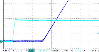
Figure 8: Turn-On Transient, at full resistive load and 100 µF output capacitance, initiated by Vin. Ch 1: Vout (5 V/div); Ch 2: Vin (10 V/div). Timescale: 10.0ms/div.
