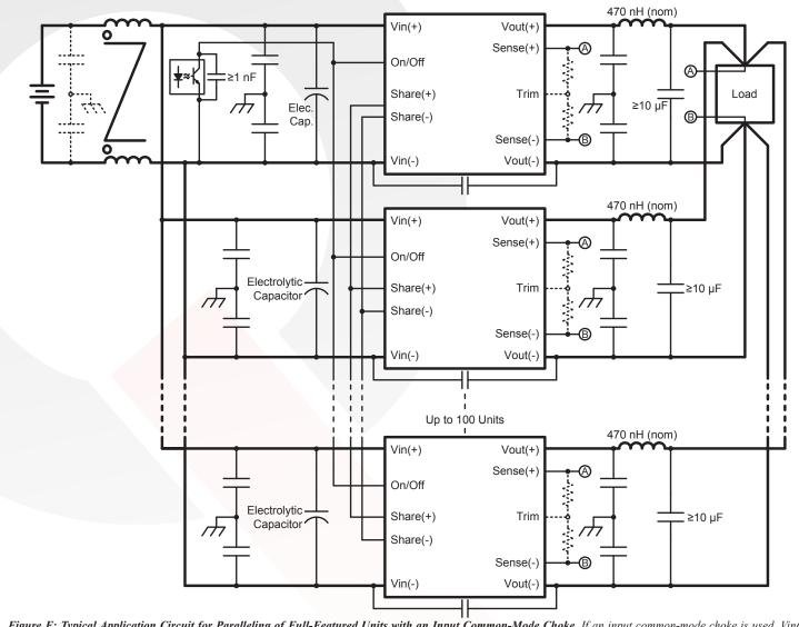
*Figure F: Typical Application Circuit for Paralleling of Full-Featured Units with an Input Common-Mode Choke. If an input common-mode choke is used, Vin(-) MUST be tied together AFTER the choke for all units.* 470 nH (nominal) inductor or an output common-mode choke is required for outputs >18 V. See Figure G for output common-mode choke configuration.
