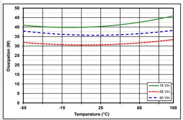
Figure 4: Power Dissipation, at nominal output voltage and 100% rated power vs. case temperature for minimum, nominal, and maximum input voltages.
