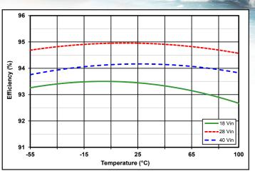
Figure 2: Efficiency, at nominal output voltage and 100% rated power vs. case temperature for minimum, nominal, and maximum input voltages.
