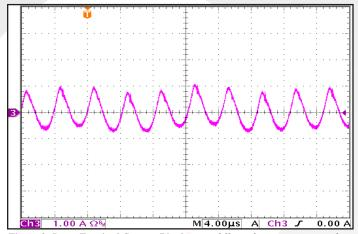
Figure 9: Input Terminal Current Ripple, i<sub>C</sub>, at full rated output current and nominal input voltage with a 100 µF electrolytic capacitor (1 A/div). Bandwidth: 20 MHz. See Figure 13. Timescale: 4.00µs/div.
